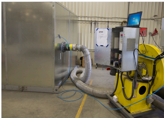
Figure 1 - Example of standard pressure test for an AHU
