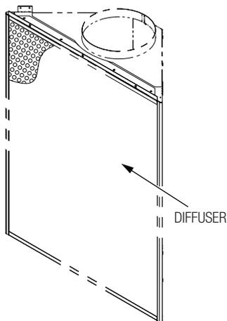
1. Bend the tabs on the duct cover caps in the upward position (Figure 1). Fasten a duct cover cap (Item 1) to the top of the displacement diffuser ensuring that the tabs are facing up (Figure 2). Fasten the mounting flange to the wall with the tabs located at the end of the flange (Figure 6).
