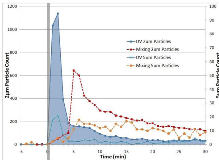
Figure 4 - Area under the concentration curve of the 2 micron particles vs. time with displacement ventilation
