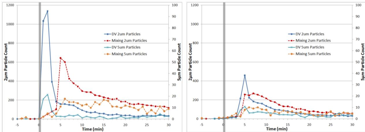
Figure 2 - Concentration of 2 and 5 micron particles vs. time for (a) particle source at the patient and counter at the caregiver and (b) particle source at the caregiver and counter at the patient
