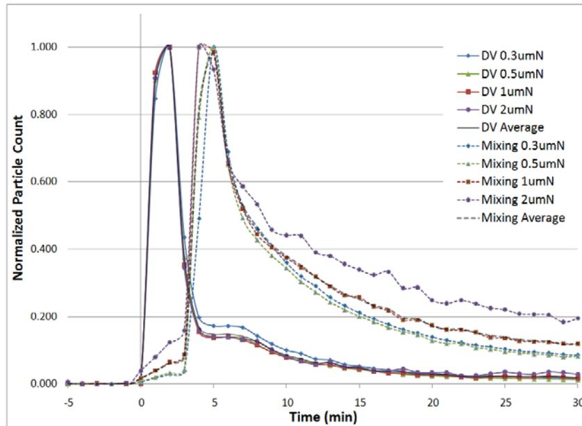
Figure 3 - Normalized particle counts for the DV and mixing systems for the case with patient source, measured at the caregiver.
