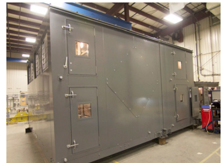
Figure 2: Example of a typical gas fired make-up air unit with HRP
