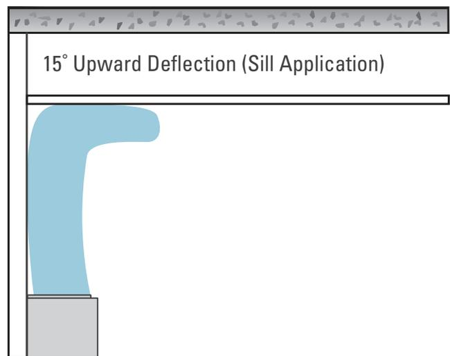
Figure 4: Floor Mounted or Sill Mounted Grill Discharging Vertically Upwards
