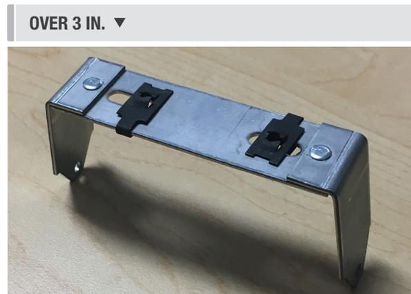
**STEP 12:** Place the outer brackets over the inner brackets, lining up the mounting screws with the black threaded clips of the outer brackets. With a screwdriver, turn each screw clockwise, alternating mounting screws to ensure that the outer bracket remains as parallel to the frame as possible. Keep turning the mounting screws until the outer brackets are approximately halfway down the length of the screws.
