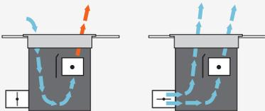
*The LFGH-RCV incorporates a heater for perimeter heating in a compact steel plenum to enclose all components. The LFGH-RCV can be ordered in multiple sections with a continuous grille to make installation easy while providing the architectural appeal of a continuous piece.*
