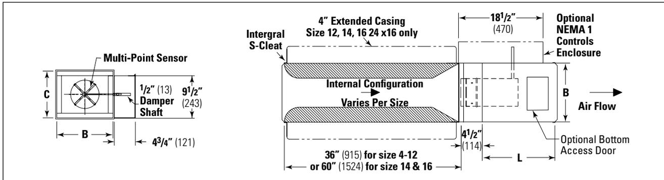
Damper rotation is always clockwise to the open position. An identification mark on the end of the shaft indicates the damper position.
