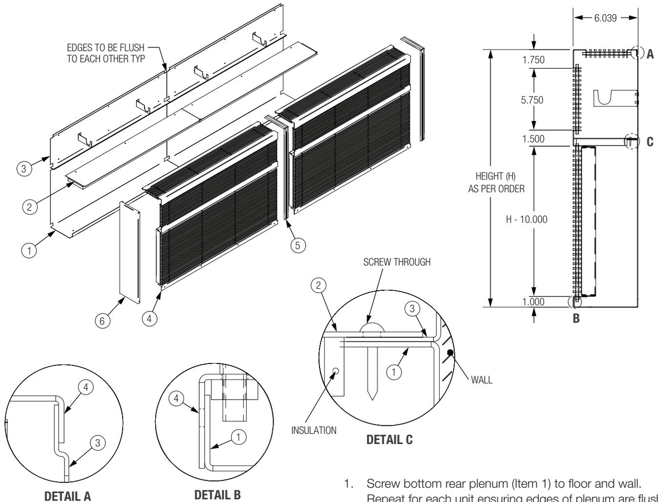
1. Screw bottom rear plenum (Item 1) to floor and wall. Repeat for each unit ensuring edges of plenum are flush to each other.
