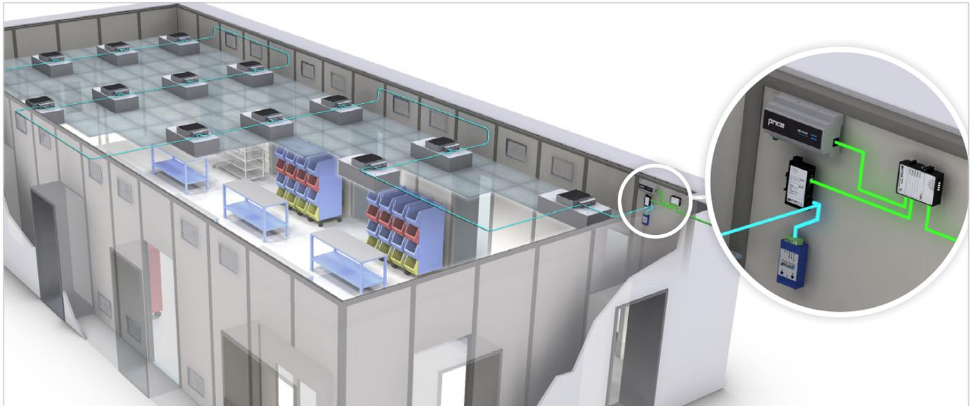
*An example of Fan Filter Units in a cleanroom on a BACnet system. The BACnet router's MS/TP port links to the BACnet Commissioning Tool and the Fan Filter Units, and the Ethernet port connects to an IP switch that services the Web Server and the building's local area network (LAN).*
