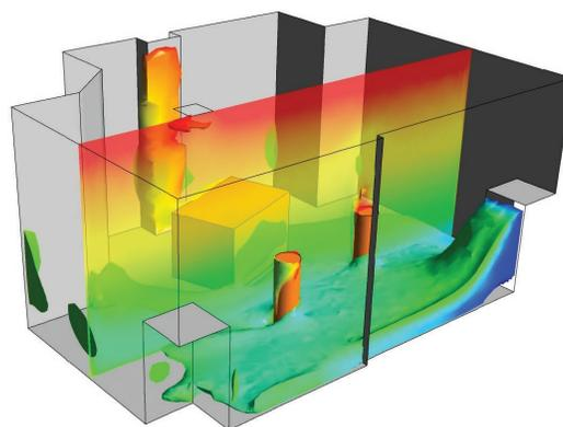
Displacement Ventilation: Stratified temperature
