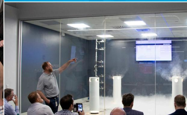
**SMOKE DEMONSTRATIONS** Using theatrical smoke, Price product performance and HVAC concepts are demonstrated for numerous products including GRD, UFAD, Chilled Beams, and Displacement Ventilation.
