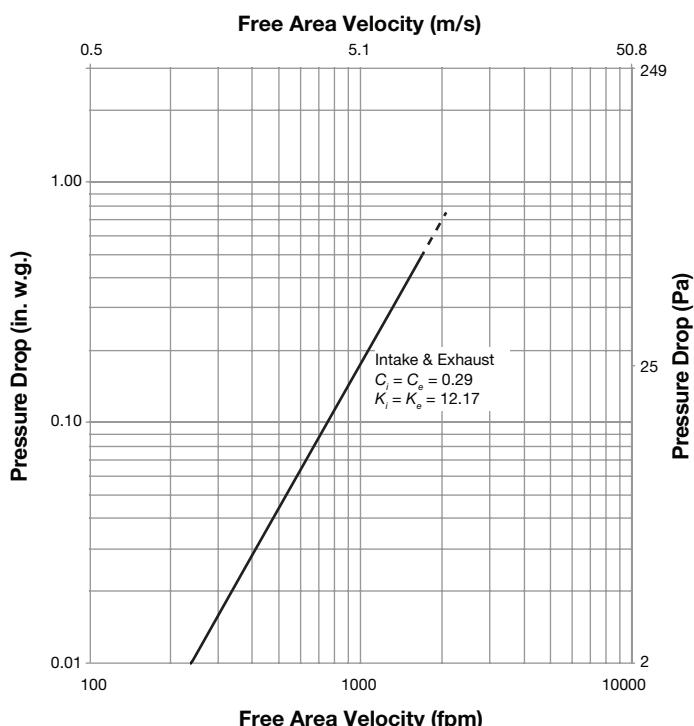
Air Performance Rating characterizes the resistance of the louver by measuring the pressure differential at various free area velocities. Intake and exhaust coefficients based on core area as per BS EN 13030.
