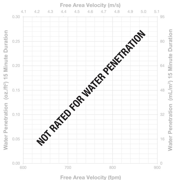
First Point of Water Penetration is the point at which a louver allows the passage of water through the louver. It is a measurement of the air intake velocity at which the louver will begin leaking.
