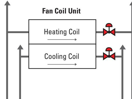
**Figure 20:** Common Coil 4 Pipe System
