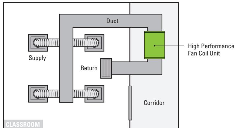
**Figure 9:** Horizontal High Performance Fan Coils
