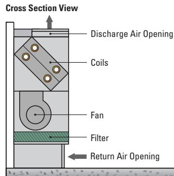
**Figure 5:** Horizontal Fan Coil Arrangement
