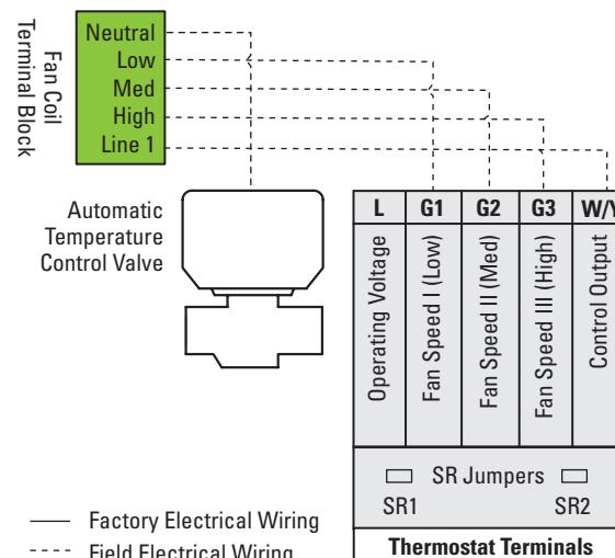
**Figure 23:** Sequence of operation for manually selected fan speed and manual heat-cool changeover
