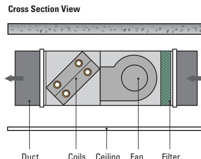
**Figure 6:** Horizontal Concealed Fan Coil
