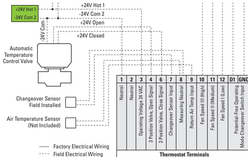
**Figure 26:** Sequence of operation for automatic heat-cool changeover and modulating control of heating and cooling
