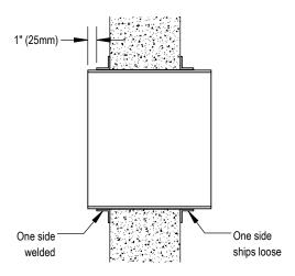
☐ MR6 - 3/4" x 3" (19mm x 76mm) Masonry rods, welded on top and bottom of sleeve, maximum 12" (305mm) on center spacing
