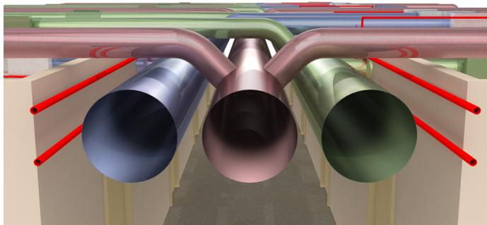
**Figure 3:** Hospital patient room hall interstitial space for an all-air system (supply duct, exhaust duct, and return duct)
