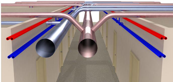
**Figure 4:** Hospital patient room hall interstitial space for an active chilled beam application (supply duct, exhaust duct, and chilled water piping)
