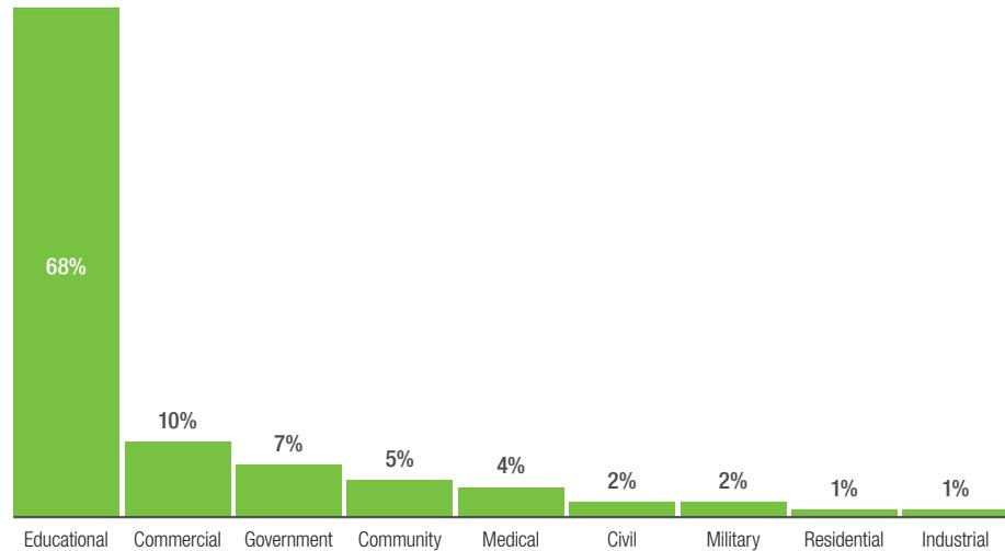
**Table 1:** Building types and percentage of total building types using chilled beams (2012 to 2014\*)
