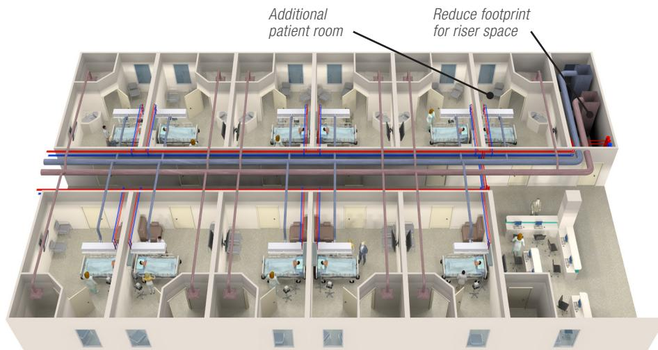
**Figure 2:** Reduced riser and mechanical room space requirements could allow for an additional patient room on each floor
