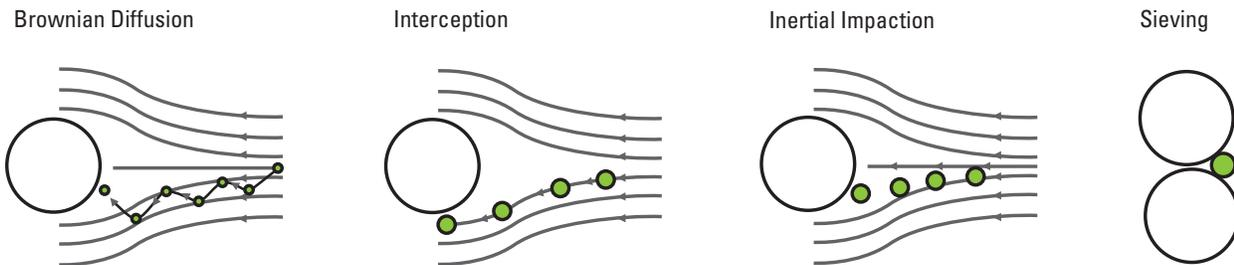
Figure 3 Filtration Mechanisms
