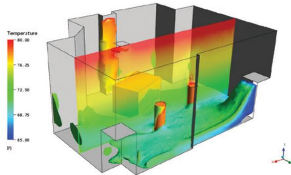
Figure 4: CFD Model of Thermal Performance
