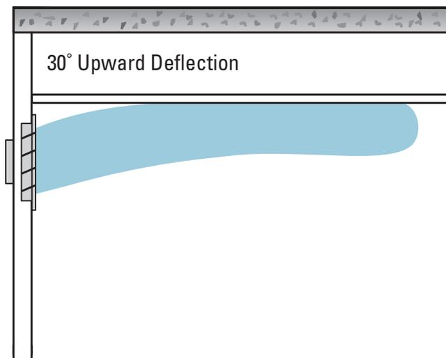
Figure 3: Sidewall Grille Mounted at High Level Discharging Horizontally
