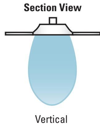
Figure 2: Ceiling Mounted Diffuser Discharging Air Vertically Downwards
