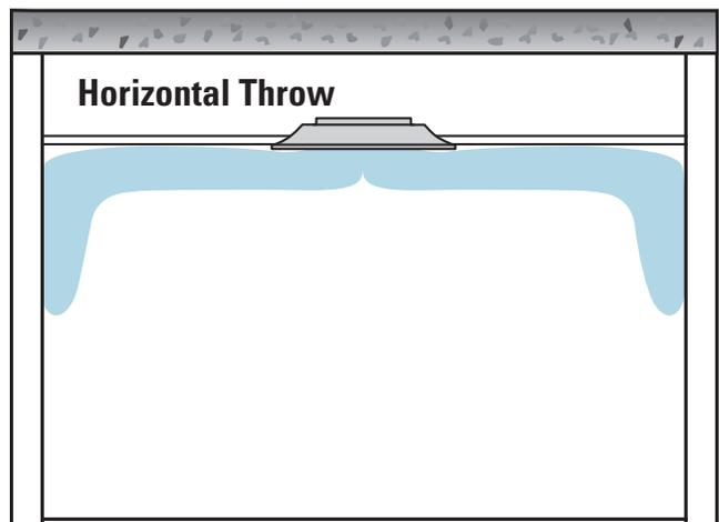
*Figure 1: Ceiling-mounted Diffuser Discharging Horizontally*
