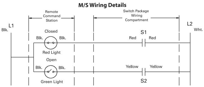
L1, L2 is a Supply Voltage Compatible with Lights and Switches. Standard Voltage is Same as Actuator Ordered.
