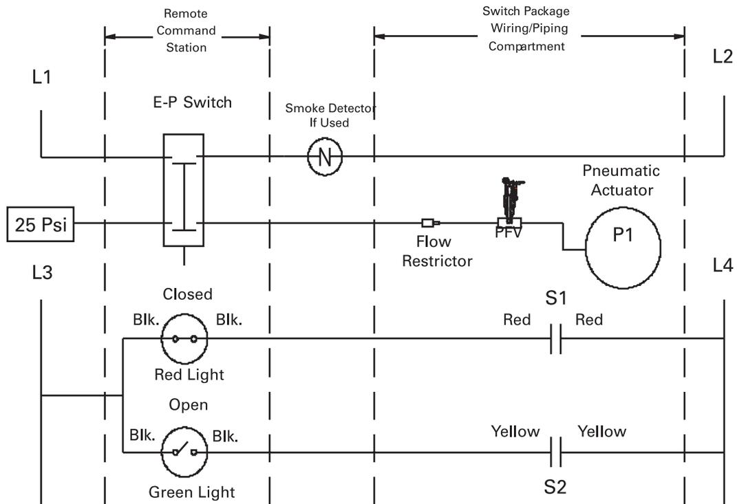
L3, L4 is a Supply Voltage Compatible with Lights and Switches. Standard Voltage is 120vac if not Specified.
