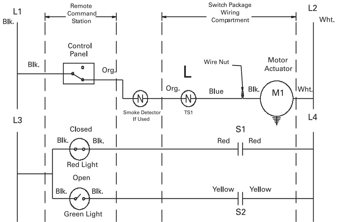
L3, L4 is a Supply Voltage Compatible with Lights and Switches. Standard Voltage is Same as Actuator Ordered.
