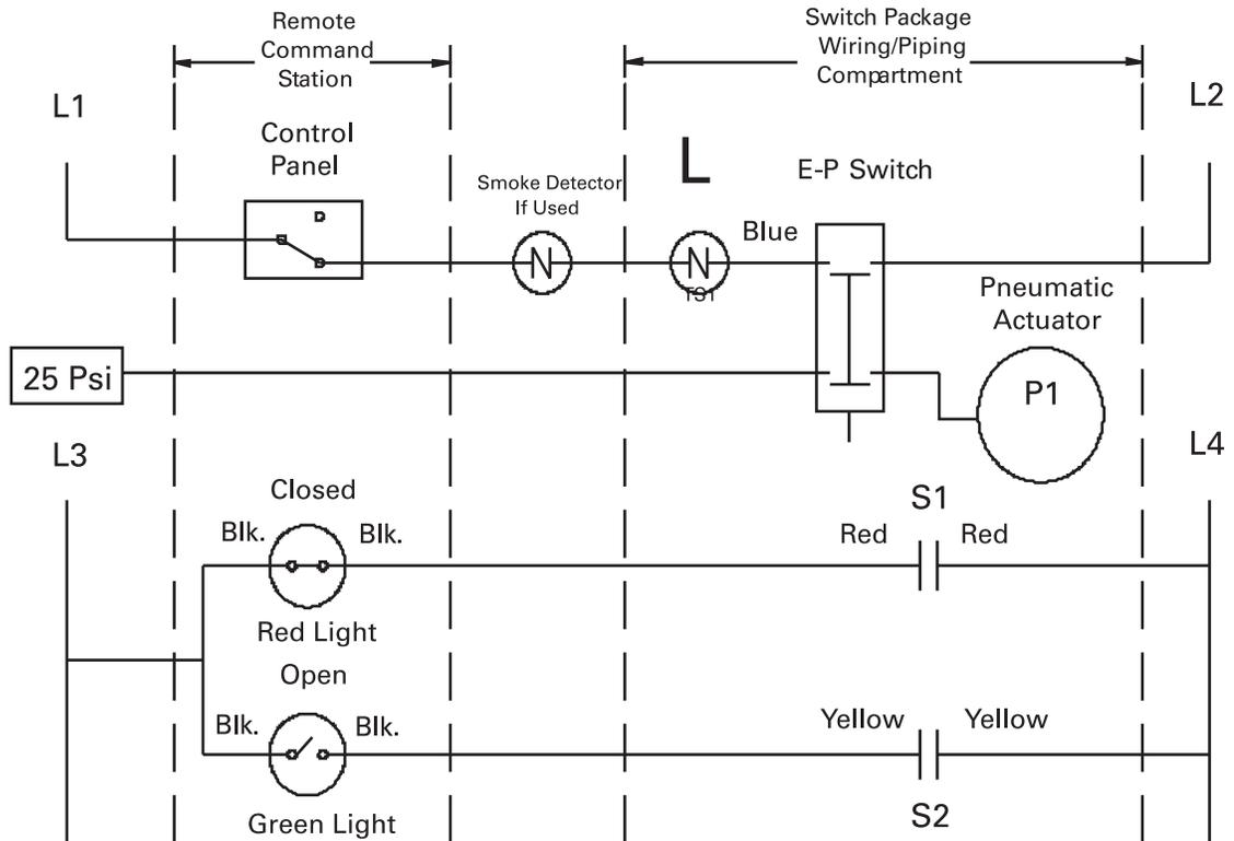
L1, L2 is the E-P Switch Supply Voltage desired (120vac or 24vac). L3, L4 is a Supply Voltage Compatible with Lights and Switches. Standard Voltage is 120vac if not Specified.
