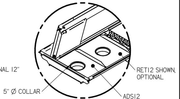
IF RETURN/EXHAUST ALSO SELECTED, RET IS BETWEEN ADS AND ACTIVE BEAM SECTION
