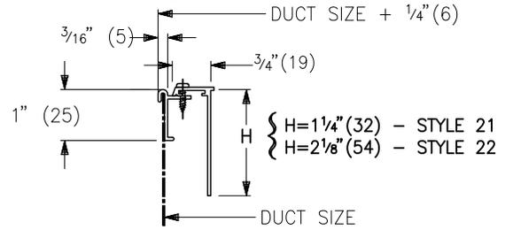
ED APPLICATION IS SUPPLIED COMPLETE WITH BORDER AND DUCT MOUNTING FRAME
