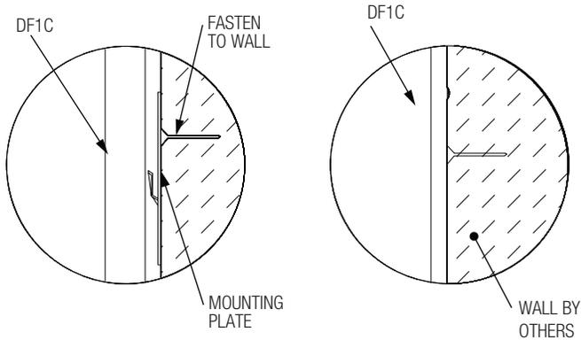
1. Fasten the mounting plate (Item 2) to the wall at the specified distance above the floor (Table 1, Figure 1 and Figure 2 for reference).
