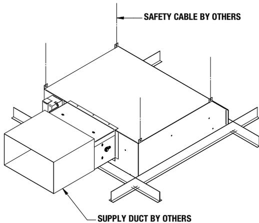
1. Fit DF1L-HC through an opening in T-bar ceiling grid at the desired location (Figure 1).
