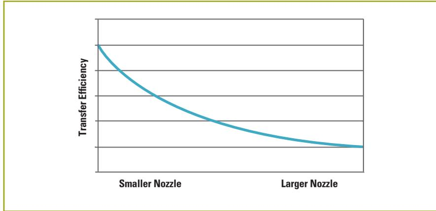
**Figure 32:** Transfer efficiency is reduced by increasing nozzle size
