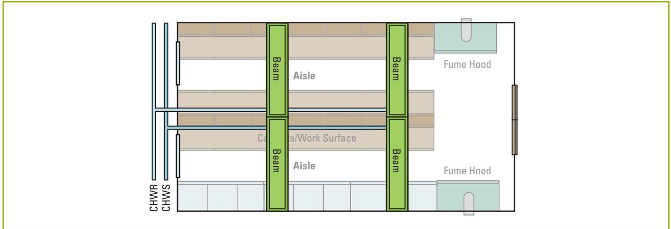
With this spacing, the 4.5 m throw to 0.25 m/s will cover the room well with 3 m of throw to the wall and opposing air pattern and 1.5 m from the ceiling to the top of the occupied zone. It is logical to run the supply and return piping down the middle of the room and have the water connections for the beams face each other, as indicated on the diagram.
