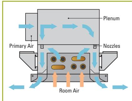
**Figure 1:** Air flow diagram of a typical linear active beam in cooling
