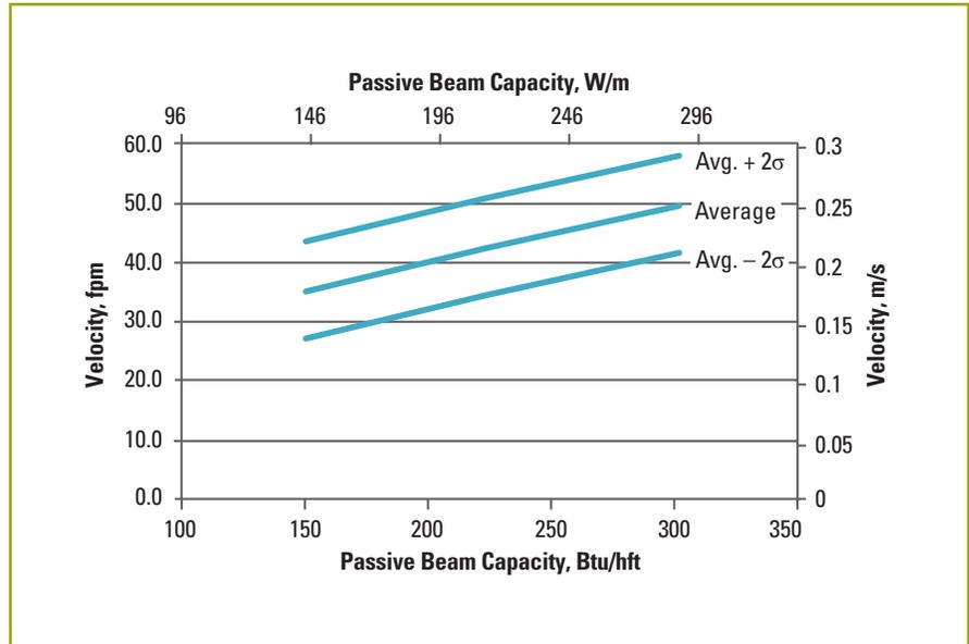
**Figure 27:** Expected velocities below an 18 in. wide passive beam
