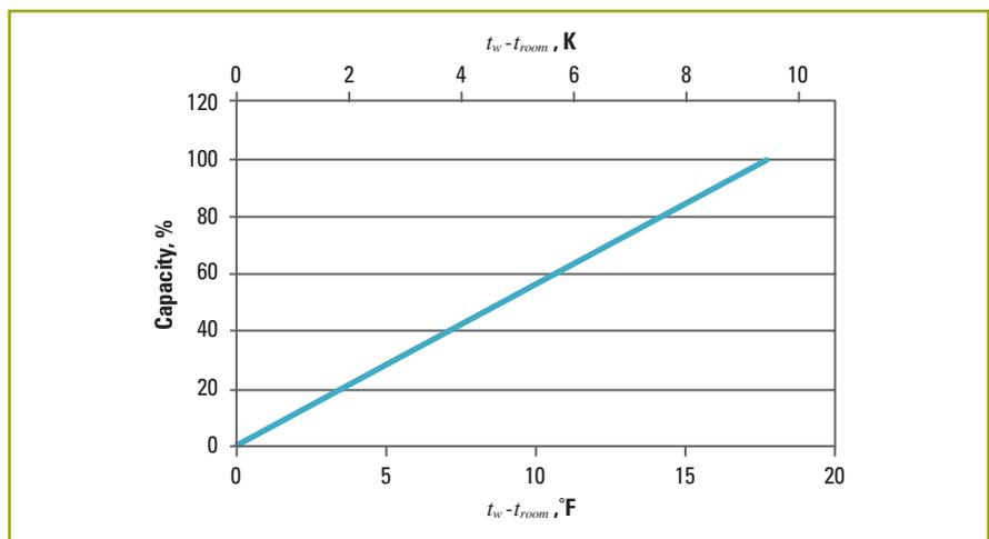
**Figure 36:** Active beam capacity vs. difference between the mean water and room air temperatures
