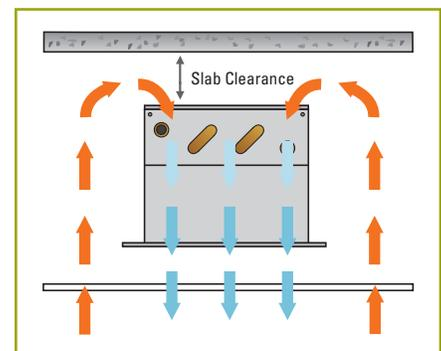
**Figure 23:** A passive beam installed above a perforated ceiling
