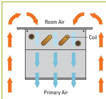
**Figure 6:** Air flow diagram of a passive beam in cooling
