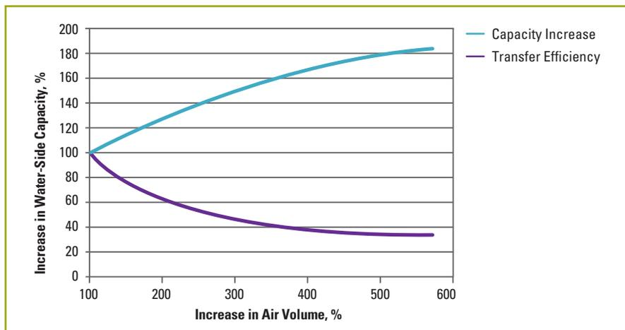
**Figure 34:** Capacity vs. air volume
