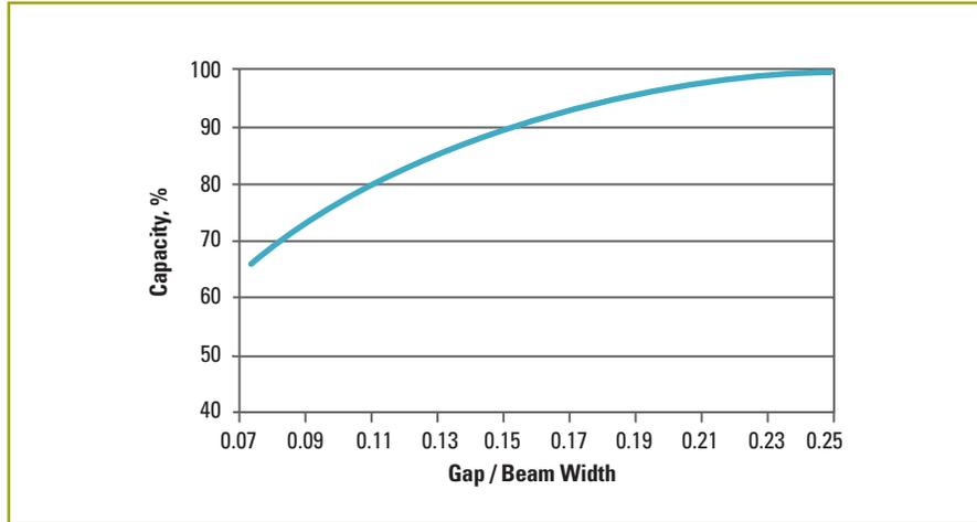
**Figure 24:** The impact on the capacity of the gap between a passive beam and building structure
