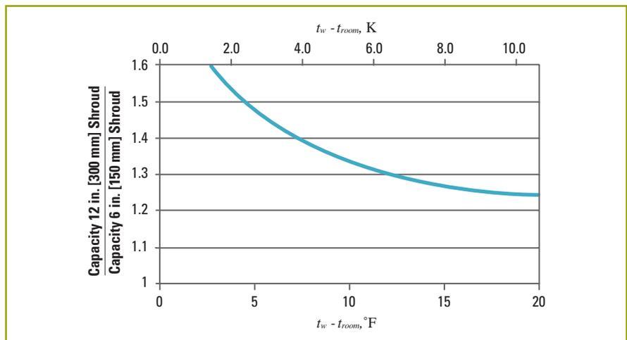
**Figure 21:** Passive beam capacity vs. temperature difference
