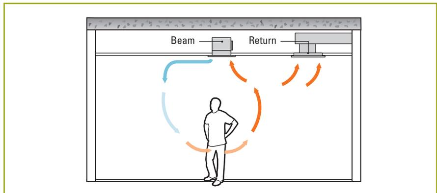
**Figure 15:** Room air flow pattern of a typical linear active beam in cooling
