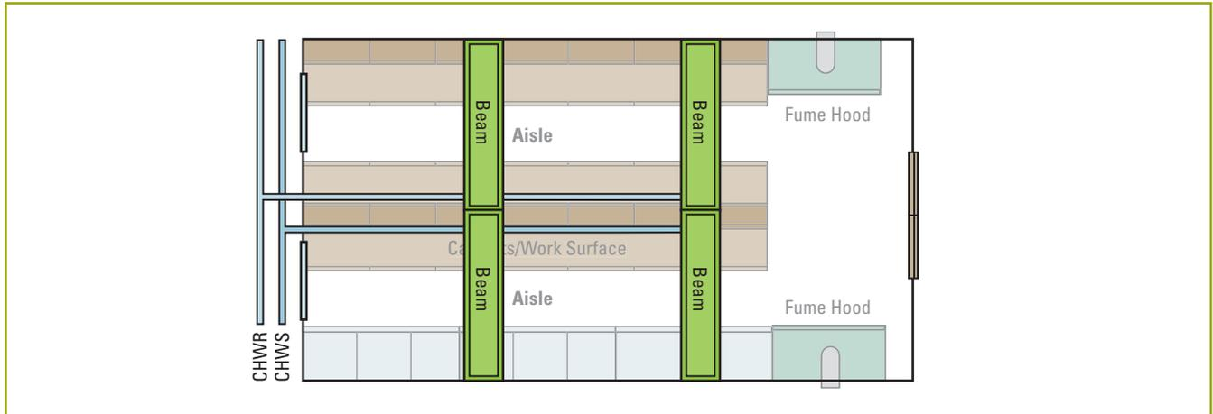
With this spacing, the 14 ft throw to 50 fpm will cover the room well with 9 ft of throw to the wall and opposing air pattern and 5 ft from the ceiling to the top of the occupied zone. It is logical to run the supply and return piping down the middle of the room and have the water connections for the beams face each other, as indicated on the diagram.
