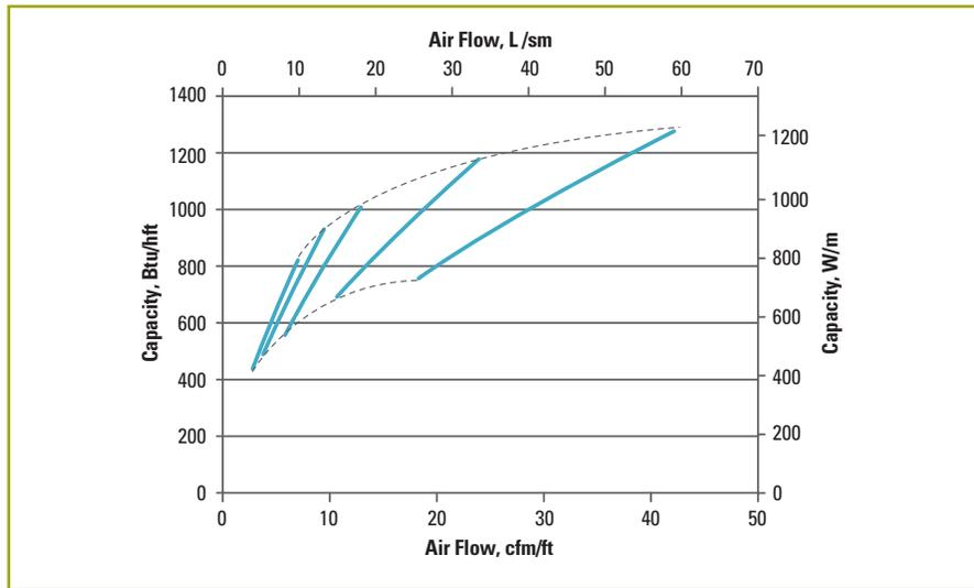
**Figure 33:** Capacity of a typical active beam vs. primary air flow
