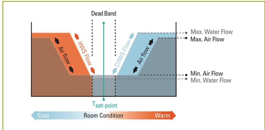
**Figure 37:** VAV control sequence
