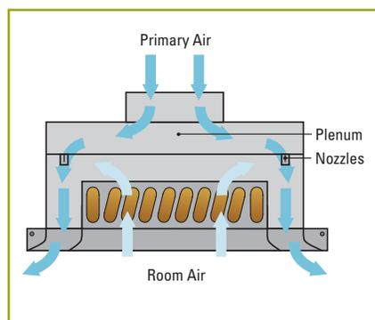
**Figure 16:** Air flow diagram of a modular beam in cooling
