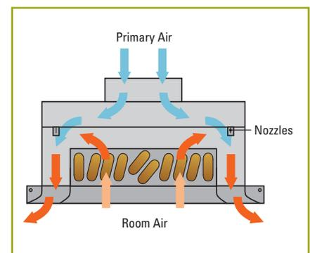
**Figure 17:** Air flow diagram of a modular beam in heating
